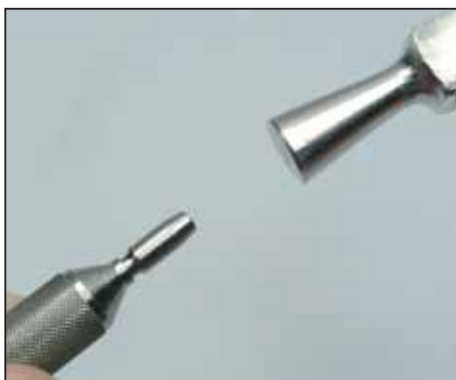
3.4 Placement of the abutment on the specific handle for holding abutment. Particular care must be taken in finding the engagement in the internal hexagon. The handle facilitates the reduction of the abutment and prevents any damages to the abutment. It also avoids problems due to overheating and unstable grips.
