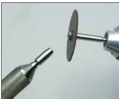
3.5 First phase of the reduction of the abutment seated on the handle. The abutments of the LEONE EXACONE™ Implant System allow an easy preparation both in the laboratory and in the patient's mouth, due to the particular quality of the titanium utilized and to their design (solid abutments). Separation disks and cross cut tungsten carbide burs are particularly indicated for this type of preparation.
